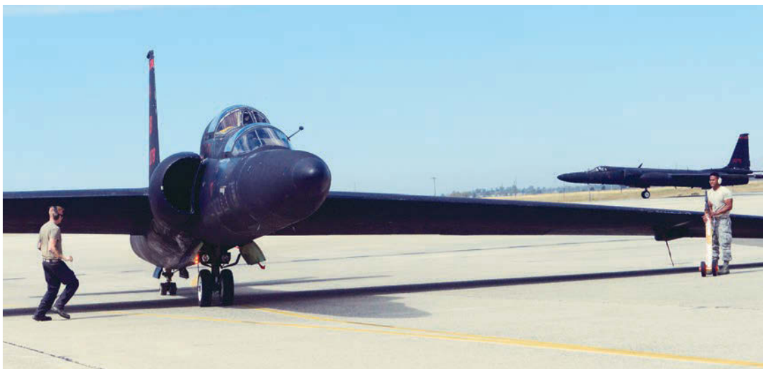
A Tu-2S Dragon Lady trainer is ready for airmen to attach "pogo" wheels at Beale AFB, Calif.
